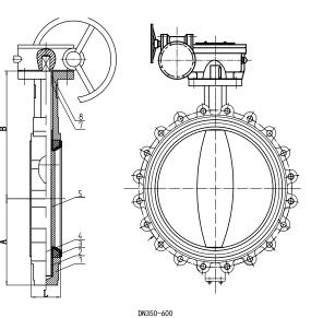
TRUEVALVE WAFER TYPE BUTTERFLY VALVEPart DescriptionMaterialBodyGGG40 Ductile IronDiscNickel-SS304 -SS316 -PTFEGasketEPDM-NBR-VITON-PTFEStuffingPTFEShaftAISI SS420
