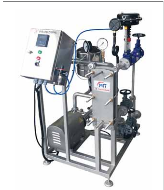
It is a hygienic complete system for foodstuff and heating liquid material. produced for a company serving in food sector.
